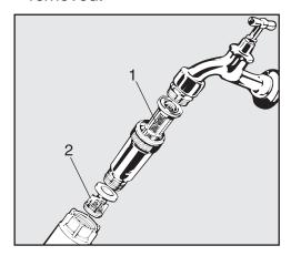
Install the filter (supplied in accessory pack) between the stopcock valve and the inlet hose. The filter for DI water is made of chromium-nickel steel and can be recognized by its dull surface and green label.
