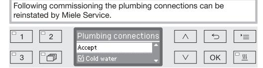
The plumbing connection is set via multiple choice. A box  $\square$  is shown in the display next to all plumbing connections. If the connection is activated, a tick  $\square$  can be seen in it. Select to activate or deactivate the plumbing connections.
