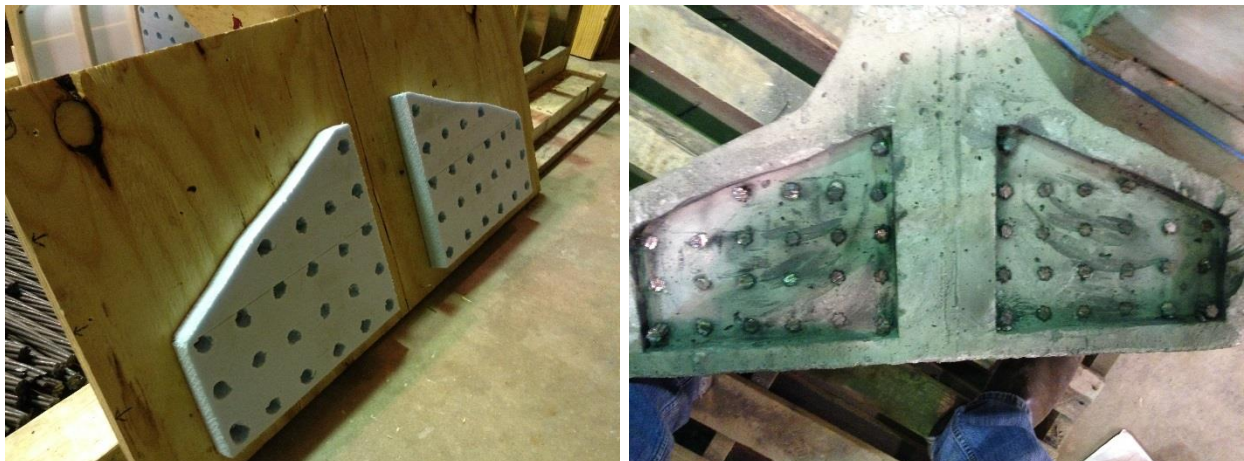
Figure 77. Double Blockout formed with 1 in. foam
