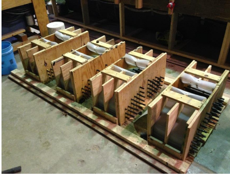
Figure 73. Formwork for laboratory beam-end specimens
