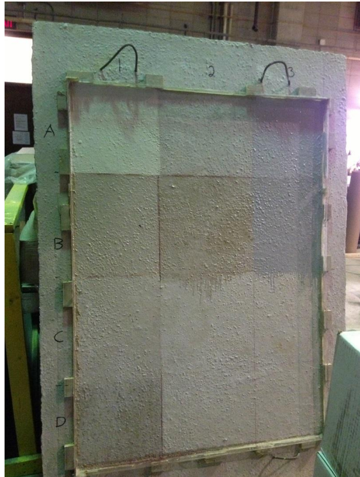
Figure 2. Typical ponding slab with coating alternatives applied
