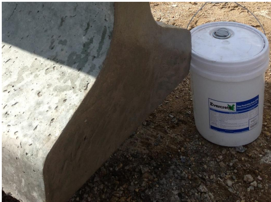
Figure 38. Evercrete DPS applied to BC11529
