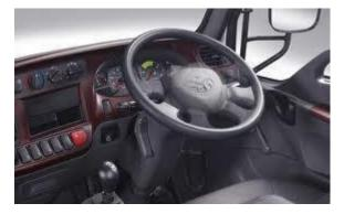
Fig: Tilt & Telescope Column
