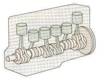
Fig: In line engine or 6 cylinder engine
