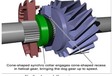
Fig: Synchromesh Concept
