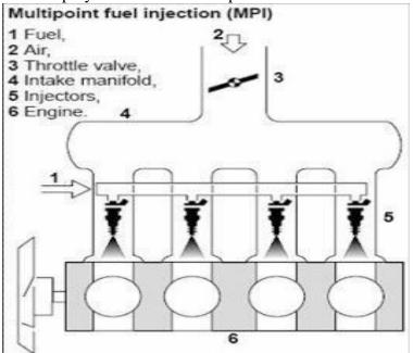
Fig: Multi-point Gasoline Fuel Injection System
