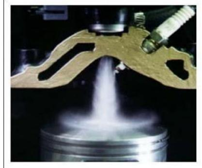
Fig:Direct Injection Gasoline Fuel System
