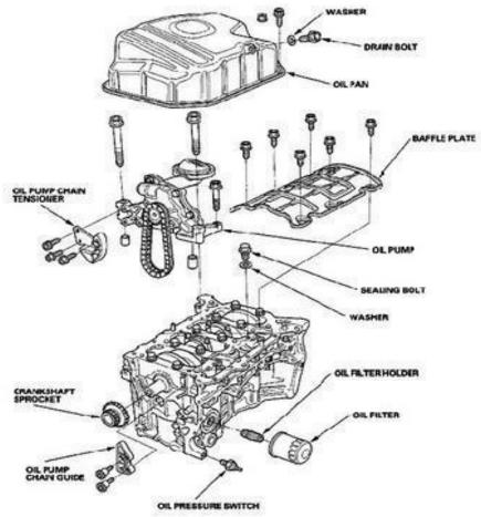
Fig: Engine Lubrication System
