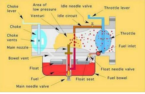
Fig: Carburetor Operation
