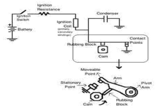
Fig: Contact Point Ignition System
