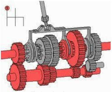
Fig: 4 speed gearbox
