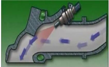
Fig: Indirect Injection Gasoline Fuel System
