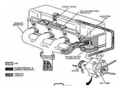
Fig: Air Injection System
