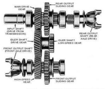
Figure – Transfer Case Gear Train in Neutral
