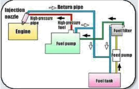
Fig: Diesel Fuel Injection System
