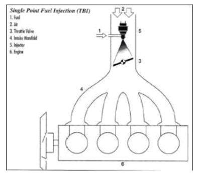
Fig: Single Point Gasoline Fuel Injection System
