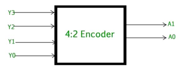
Fig: Logic Diagram of 4 : 2 Encoder The Truth table of 4 to 2 encoder is as follows :
