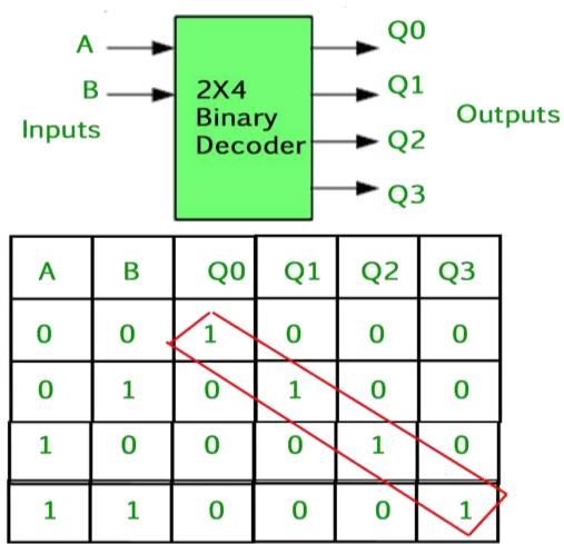
Fig: Logic Diagram and TRUTH TABLE of DECODER
