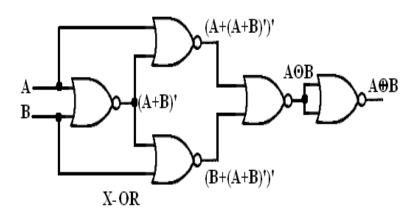
Figure-20: NOR gates as Ex-OR gate
