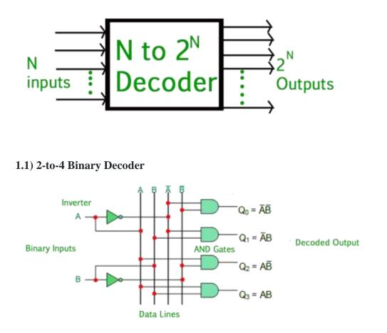
The 2-to-4 line binary decoder depicted above consists of an array of four AND gates. The 2 binary inputs labelled A and B are decoded into one of 4 outputs, hence the description of 2-to-4 binary
