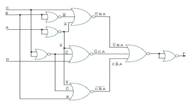
Figure-22: Implementing the simplified function with NOR gates only
