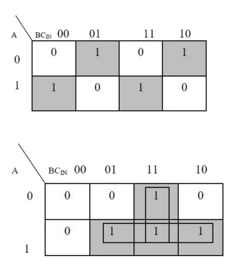
The simplified equation for sum is S = A'B'Cin + A'BCin' + ABCinThe simplified equation for COUT is COUT = AB + ACIN + BCIN
