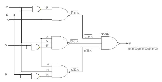
Figure-11: Implementing the simplified function with NAND gates only
