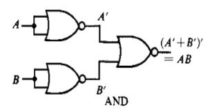
Figure-16:NOR gates as AND gate
