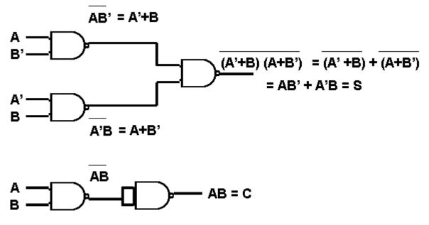
Realization of half adder using NAND gates
