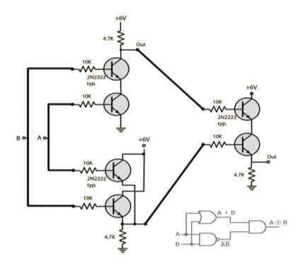
Figure-18: Ex-OR gate through RTL Logic.
