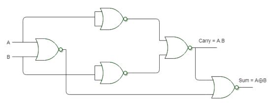
**Realization of half adder using NOR Gates**
