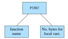
Figure 14.1: The logical structure of a function tree
