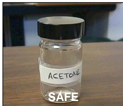
Properly labeled secondary storage container
