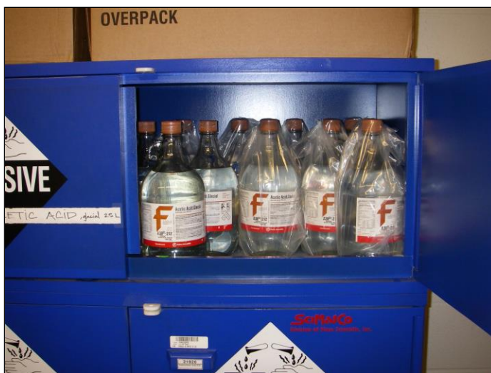
Acids stored in acid storage cabinet
