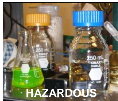
Improperly labeled secondary storage container
