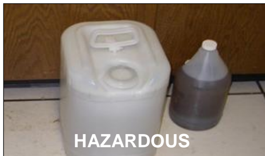
Waste container without proper identification
