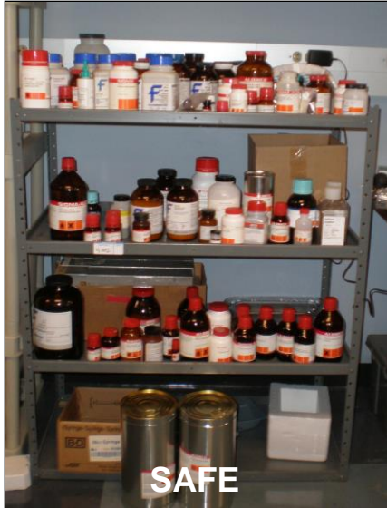
Proper storage of chemicals below eye level
