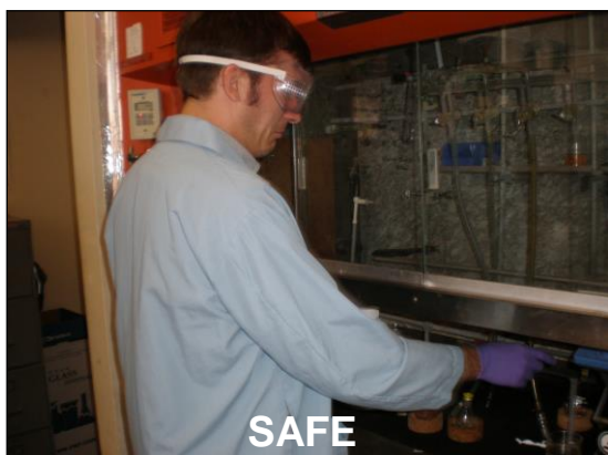
Work with the fume hood sash down as far as practical
