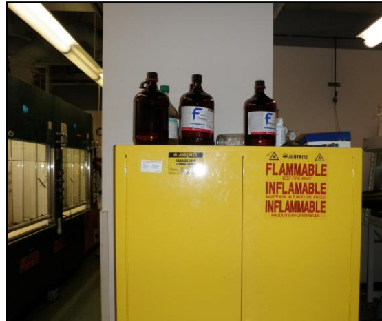
Improper storage of chemicals above eye level
