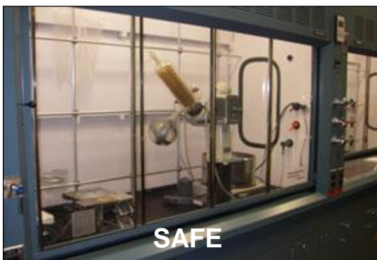
Proper use of a fume hood
