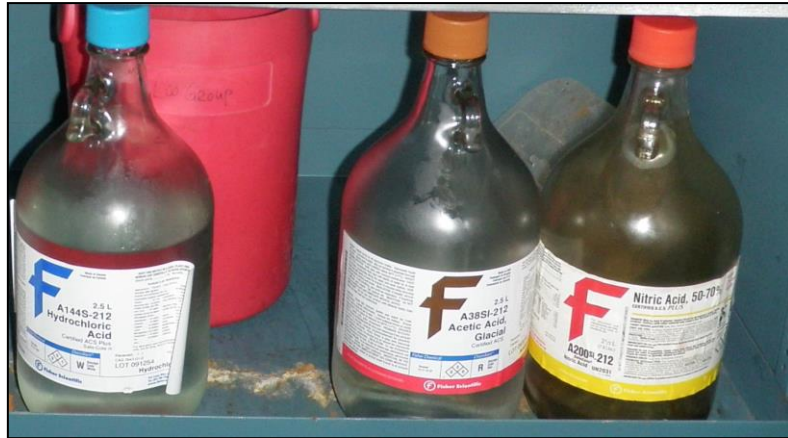
Improper storage of nitric acid
