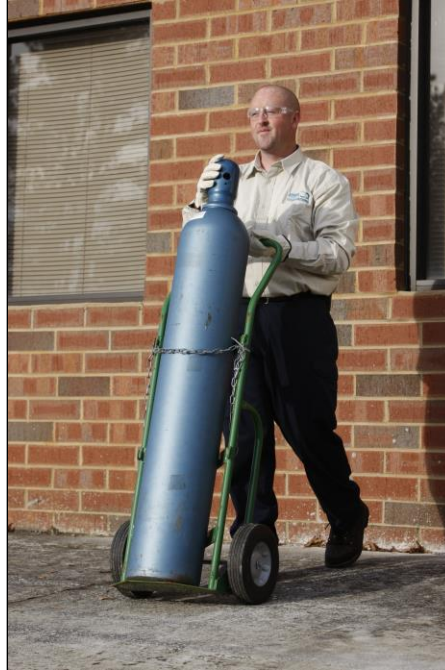
Proper transport of a gas cylinder (Picture courtesy of Airgas, Inc.)
