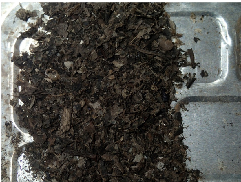
Figure 7: An image of the dried macroscopic organic detritus prior to being crushed into finer particles for use in the experiments. For scale, the rectangular indentation in the aluminum pan at the top right of the photo has a vertical dimension of 2.3 cm.
