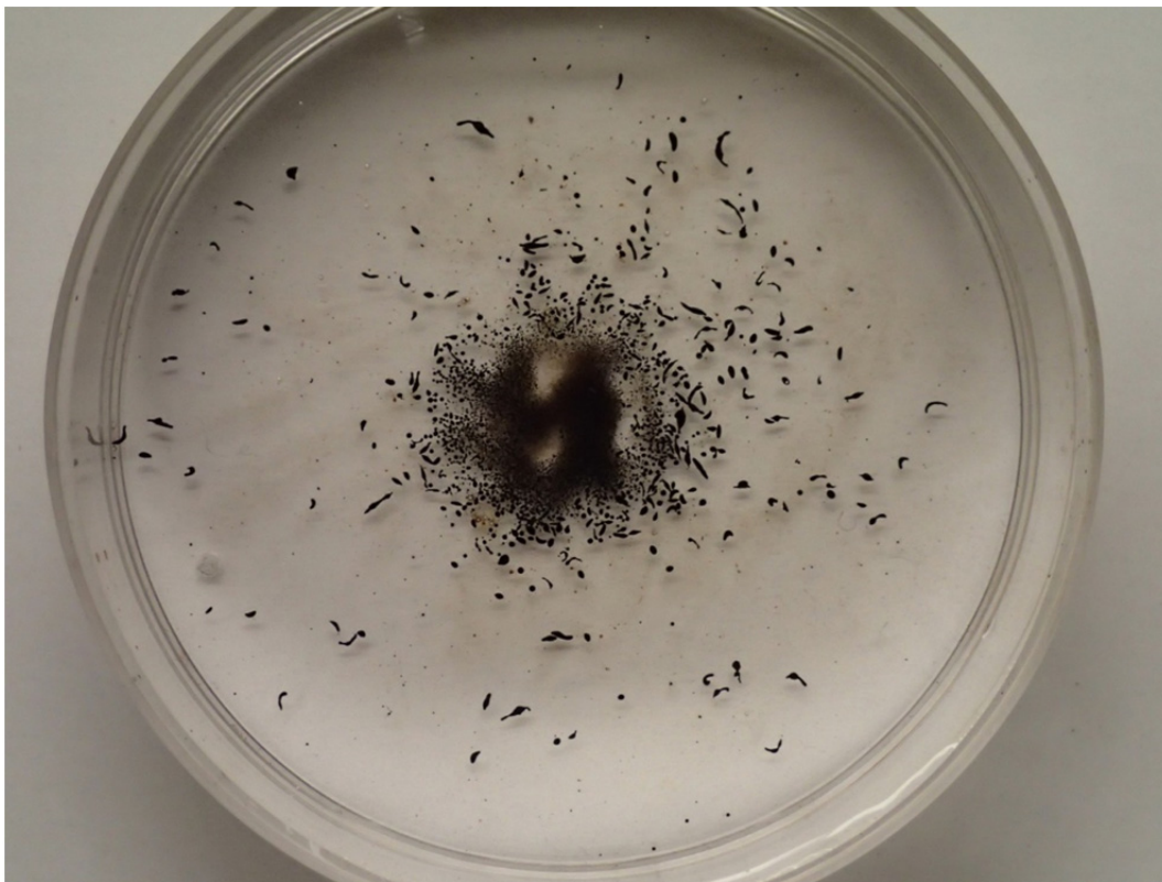
Figure 66: A view of the solid-type OPA used in the annular flume experiment. The sample is in a 60-mm diameter Petri dish. The maximum dimension of the largest OPA shown is approximately 2.5 mm.
