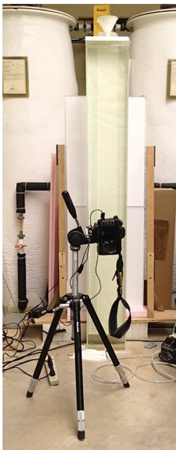
Figure 41: The settling column used for the settling velocity tests. The vertically mounted panels behind the column are LED light panels.
