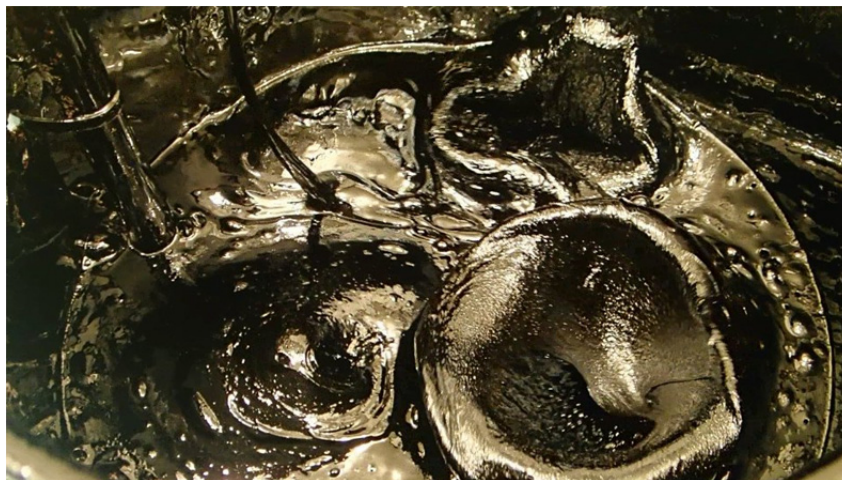
Figure 1: A frame captured from video recorded approximately 4 days into the initial oil weathering; the rigid vertical member is the CPVC air input line; the flexible line to the right of it is the temperature sensor.
