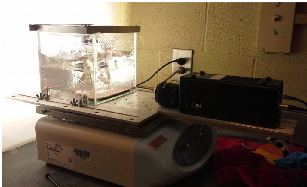
Figure 40: The setup for the photographic analysis; the baffled flask is mounted inside a small aquarium containing water to minimize optical distortion associated with the irregular flask geometry; the PIV camera rotates with the entire assembly. Lighting is provided from the rear.
