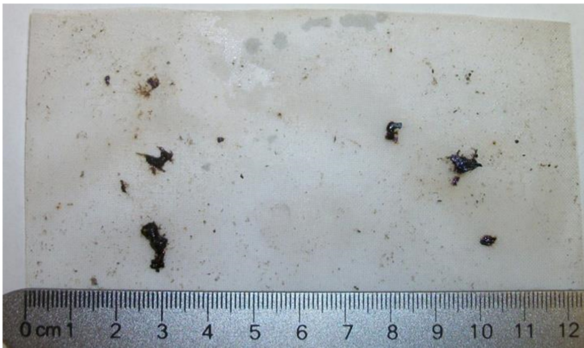
Figure 20: Large masses of sediment-laden tarry oil resuspended from the bed during fall 2014 dredging and captured from below the water surface with a sheen net. The large features were confirmed to consist predominantly of oil using UV epifluorescence microscopy. The samples were collected and photographed by Rex Johnson of GRT.
