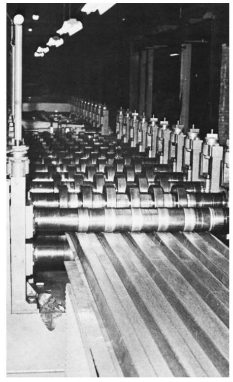
Figure 1.23 Cold-roll-forming machine.
