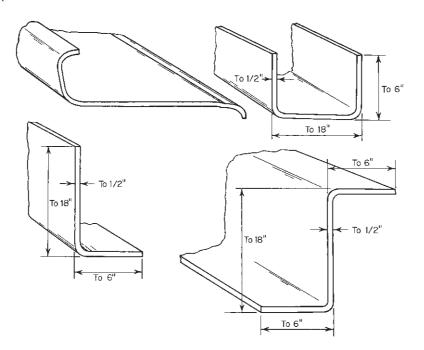
Figure 1.24 Size ranges of typical roll-formed structural shapes.<sup>1.1</sup>
