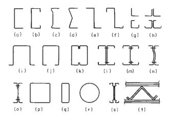
Figure 1.2 Cold-formed sections used in structural framing.<sup>1.6</sup>
