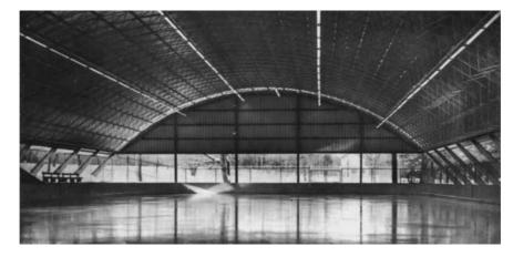
**Figure 1.8** Cold-formed steel members used in a  $100 \times 220 \times 30$ -ft  $(30.5 \times 67.1 \times 9.2$ -m) triodetic arch. (Courtesy of Butler Manufacturing Company.)
