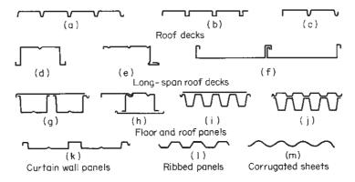
Figure 1.11 Decks, panels, and corrugated sheets.
