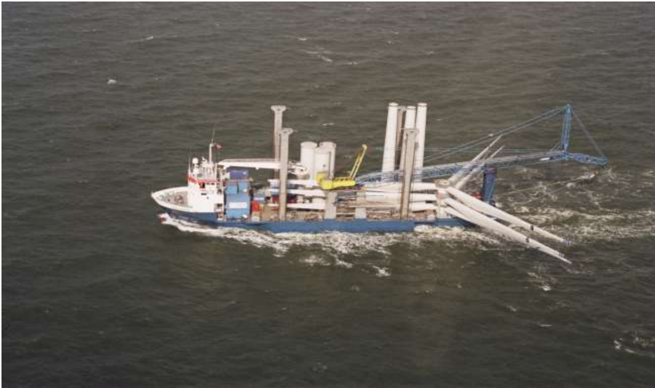
Heavy-Lift Wind Construction Ship aids in construction of Horns Rev 2 in Denmark. Photo credit: Chris Wisseman
