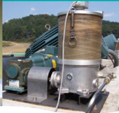
Reservoir with Low Level Switch
