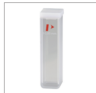
Macro Cell with PTFE Lid, Quartz SUPRASIL (B0631007)
