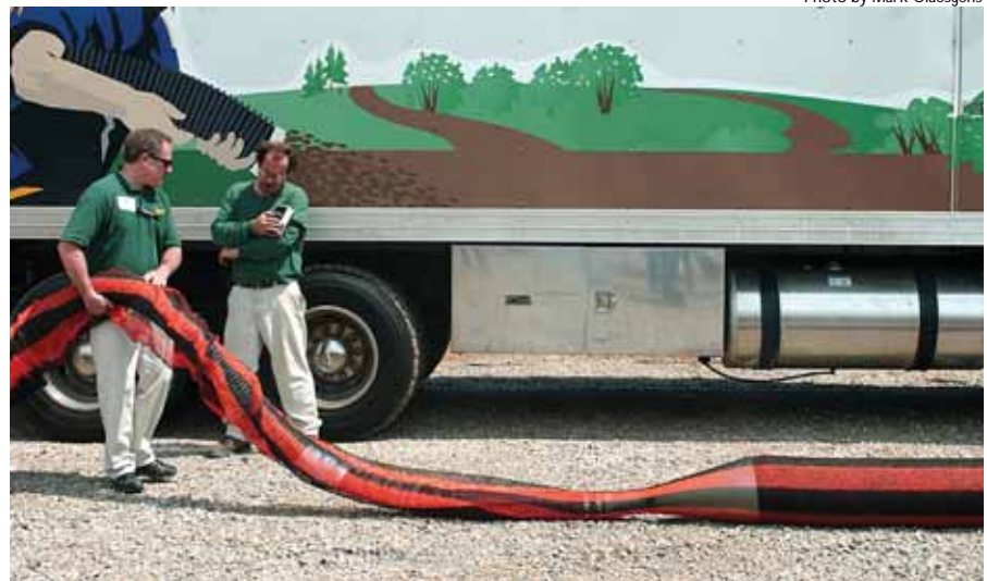
Rod Tyler (left) of Filtrexx International LLC of Grafton, Ohio, pumps a special compost mix into a "sock" while Robert Dodds of Bob's Tree Preservation of Church Point, La., which prepared the compost, monitors the flow. Once filled, the sock can be placed to filter sediment from storm water or to help erosion control. These new uses of compost were introduced at the LSU AgCenter's Callegari Environmental Center in Baton Rouge.
