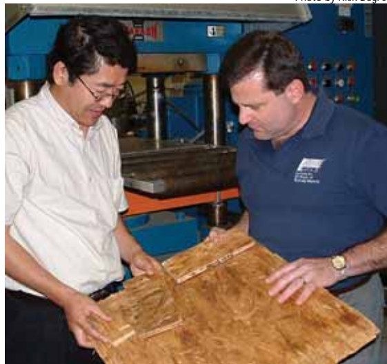
Qinglin Wu (left) and Richard Vlosky examine a piece of oriented strand board (OSB), which is composed of 50 percent sugarcane rind. The researchers say it is significantly stronger than OSB made from wood alone.
