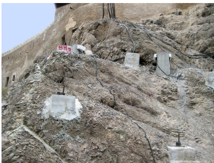
Borehole extensometers and in-place inclinometers installed for online slope monitoring at Al Mirani Fort, Oman
