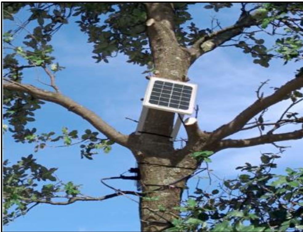
Rajah 2.9 : Waspmote Plug & Sense . (Sumber : Libelium, 2012)
