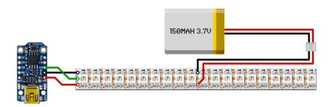
Gemma is even easier. There's already a JST connector on this board, so clipping a plug off a battery extension isn't needed. Just connect – (minus) on the strip to GND on Gemma, + to Vout, and the remaining pin to D1.
