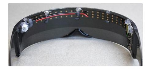
To prevent accidental contact with skin (which is slightly conductive, especially if damp with perspiration), the back side of everything is covered with tape.
