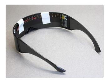
The electronics can be held in place temporarily with masking tape while a more permanent bond is arranged...
