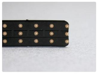
Optional: I'm not comfortable with little sharp points right next to my eyes. The strip will certainly hold in place when installed, but as an extra precaution the corners were rounded slightly at both ends of the strip. Just in case.
