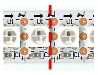
If using the high-density strip (144 LEDs/meter), you might choose to cut just to the left of the marked cut lines. When using the remainder of the strip in another project, this makes it easier to connect wires to the input.
