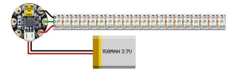
With the glasses we built upon, Trinket fit perfectly turned 90 degrees with respect to the strip (like the wiring diagram above) — the USB connector is then accessible along the top edge, for loading new code. But every pair of shades will be different. You'll probably want to use longer wires between the Trinket and strip, so you have more options when folding the pieces together; I just got carried away here with the ultrashort wires.
