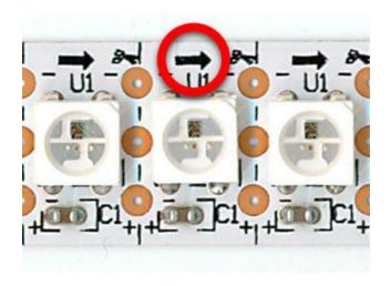
NeoPixel strip has a definite "in" and "out" end. Look for the arrows — these indicate the direction of data from the microcontroller, moving from in to out.
