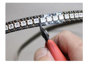
Flush cutters work well for cutting the strip. You might need to make two cuts to cover the full width; one from below, one from above.
