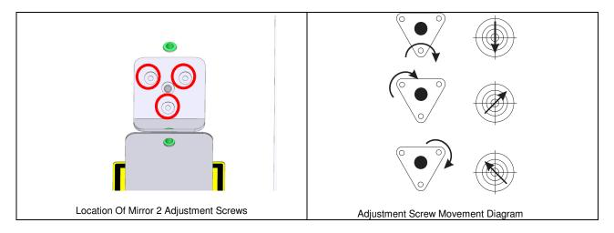
Once complete return to [Step 3]. Continue to align Mirror #1 and #2 until you can jog between them without the Red Dot leaving the Center of the alignment target.
