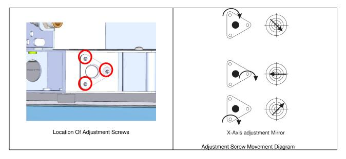
Once complete return to [Step 3] and then [Step 5]. Continue to align Mirrors #1, #2 and #3 until you can jog between them without the Red Dot leaving the Center of the Alignment Target.
