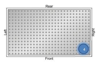
If all of the mirrors are aligned correctly, the red dot pointer should appear within the center ring on the alignment target. If so; you may remove the alignment target, replace the panels and run a test engraving file. If not; please return to [Step 3] and continue alignment.
