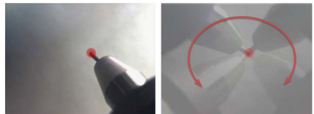
Fig. 3 Alignment of the laser focal point, the wire tip and the center of rotation stage
