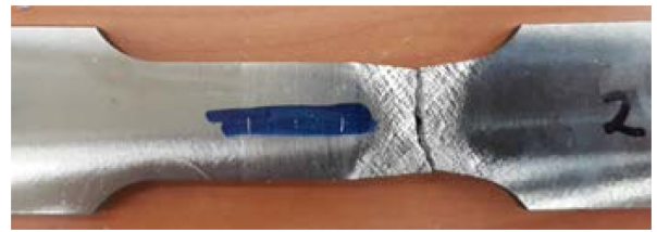
Fig. 17 Specimen fracture outside deposition and contact area
