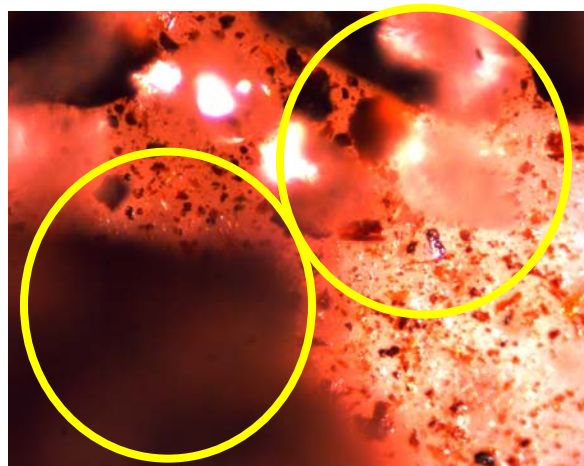
Figure 4-7. Microscope images of three soils to illustrate heterogeneity. The yellow circles represent the ablation area of the focused laser beam, approximately 0.35 \text{ mm}^2 . (Note: the 10X magnification are not the same areas as the 4X magnification areas)
