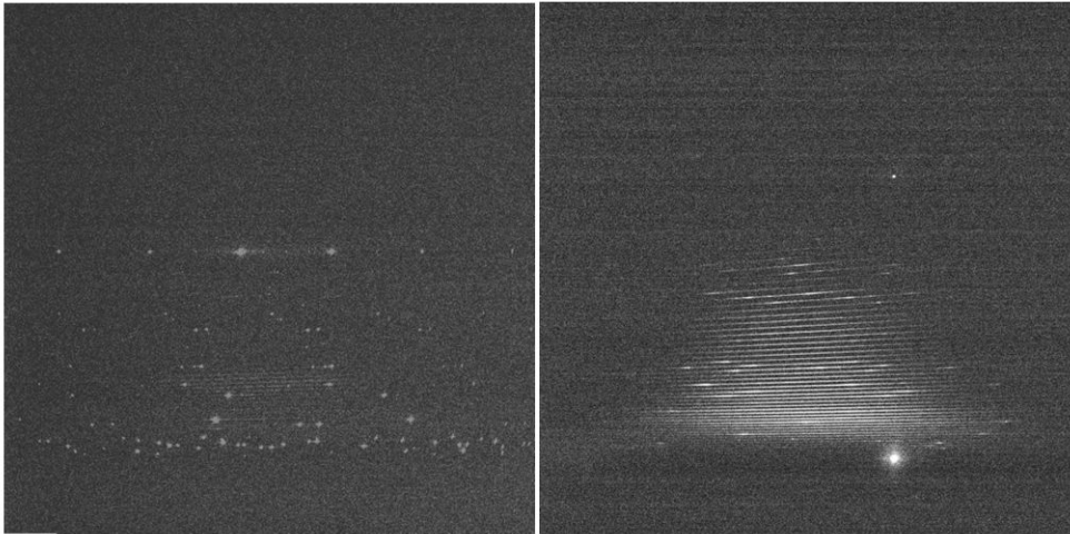
Figure 10. Echelle spectrometer dispersion image (a) Hg lamp, (b) LIBS spectrum of Sn metal
