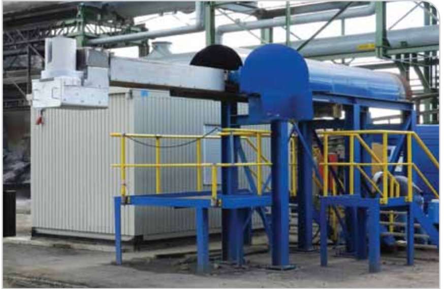
System consisting of laser head, manipulator, platform, container with equipment and operator terminal.
