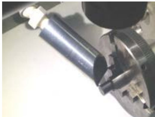
Figure 49 – Tube promoting laminar flow of argon
