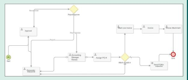
Actions performed by people, such as "Assign PO #" are represented by user tasks, actions performed by automated tools such as "Sent PO # to Requestor" are represented by service tasks and routing decisions are represented by gateways.
