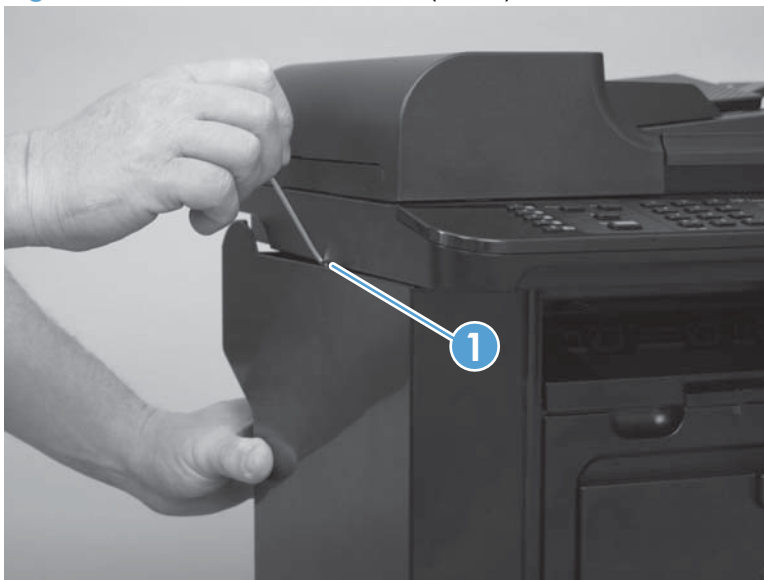
Figure 1-15 Remove the left cover (4 of 5)
