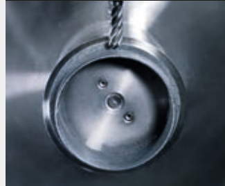
3: 90° swivel: Milling of the plane surface and the outer contour
