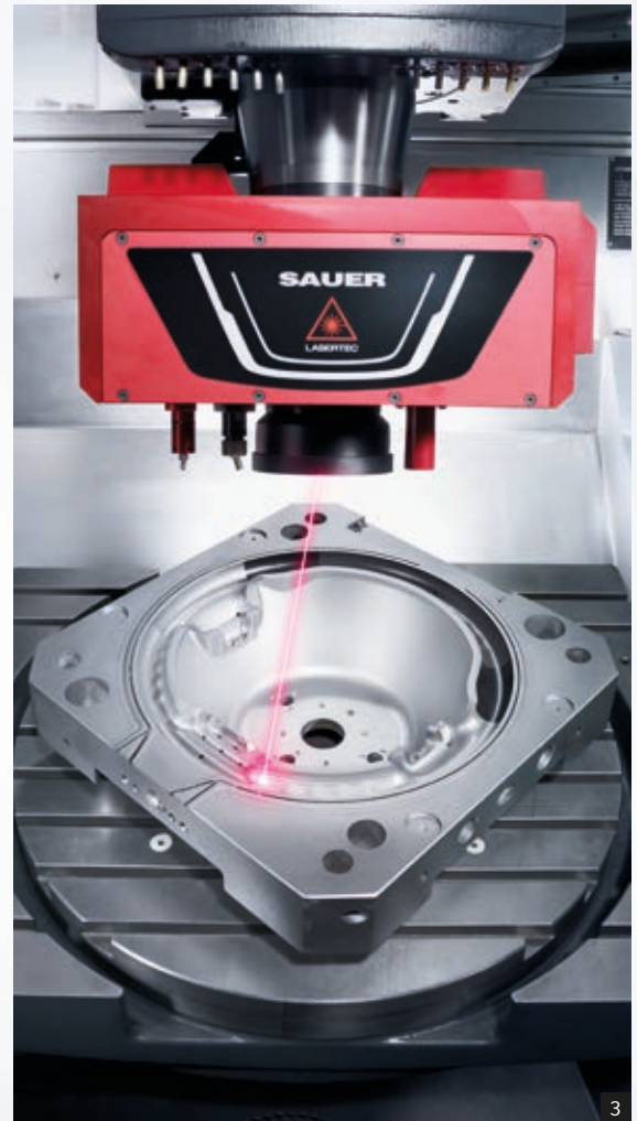
1: Large working area with integrated NC swivel rotary table with perfect accessibility, can be loaded from above by crane 2: Highly stable, compact monoBLOCK® design 3: Flexible integration of a laser scanning head via an HSK interface on the spindle, 5-axis laser texturing of a steering wheel injection mould
