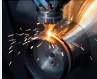
2: 90° swivel: Generation of the flange
