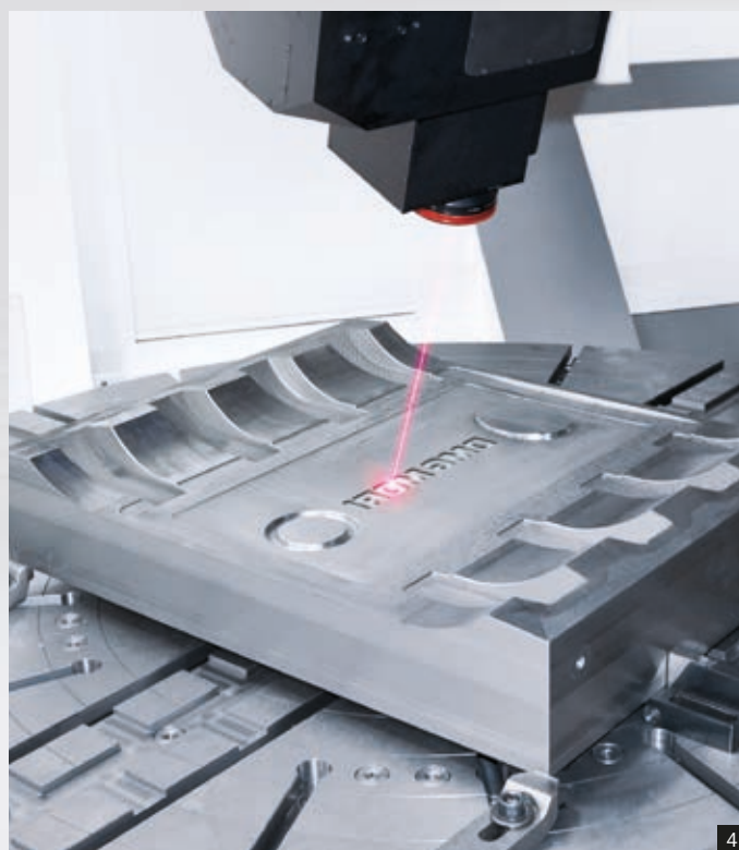
1 + 2: Replacement of the laser scanning head via a special changer device within 10 minutes; interface is the HSK 63 / 100 taper of the spindle 3: Laser texturing of a housing component 4: Surface structures in engine covers
