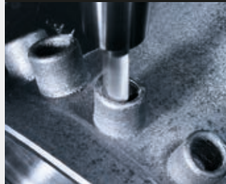
10: Milling of the connectors
