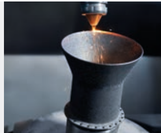
7: Laser construction of the conical funnel
