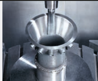
11: Milling of the flange and the inner contour
