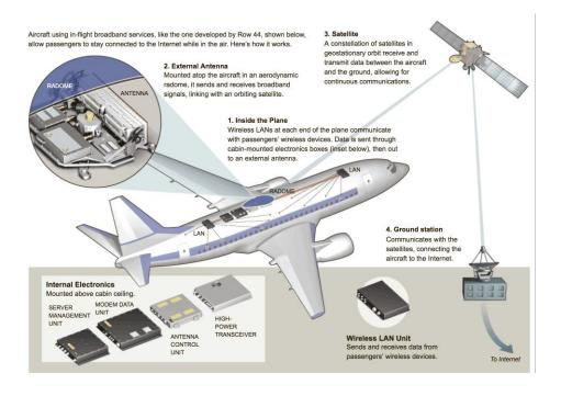
Figure 1. Basic architecture of a Row44 deployment (New York Times) 2
