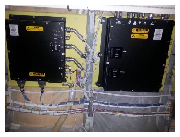
The SMU also provides the switching of data from various peripherals located in the aircraft cabin and utilizes an aircraft digital computer interface to receive aircraft position, state of flight, etc. The SMU also receives aircraft level discrete inputs to detect various conditions, including the Weight-on-Wheels signal.
