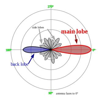
We are describing cyber-physical attacks, using compromised SATCOM antennas, assuming the main lobe is illuminating the target at a distance 'd', which is located in the Far-Field. In this region, the antenna radiation pattern is fully formed, and does not depend on the distance any more, but on the antenna's azimuth and elevation angles, which as we have seen can be controlled.
