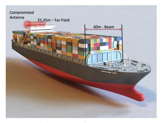
In this scenario it is also important to note that final power density values can be incremented due to the vessel design factors, which may cause resonance during the propagation.
