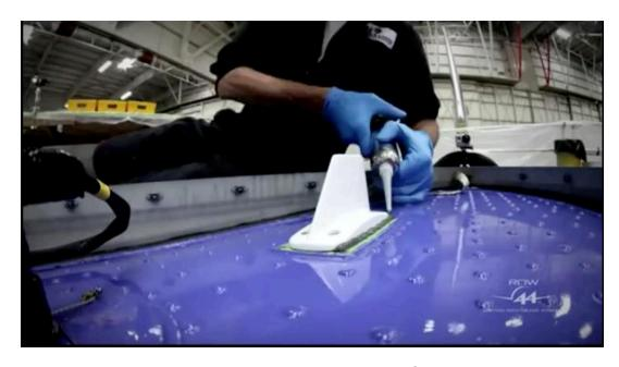
Figure 4. Cellular antenna in radome9
