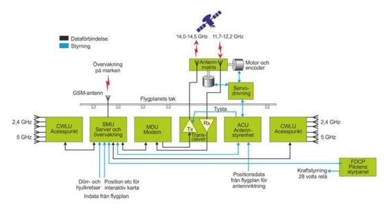
Figure 2. Detailed Row44 architecture (IDG)
