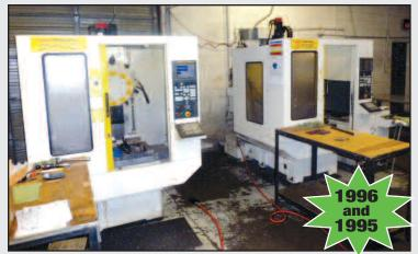
View of Fanuc Robodrill Drilling & Tapping Centers
