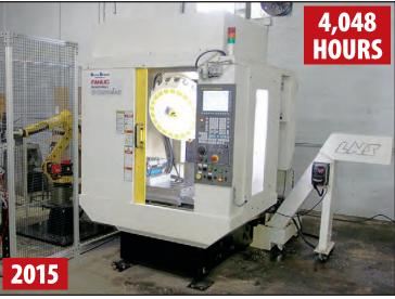
ROBODRILL A-D21MIA5 CNC VERTICAL MACHINING CENTER W/ FANUC 6-AXIS ROBOT
