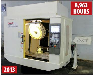
FANUC ROBODRILL A-D21LIA5 CNC VERTICAL MACHINING CENTER
