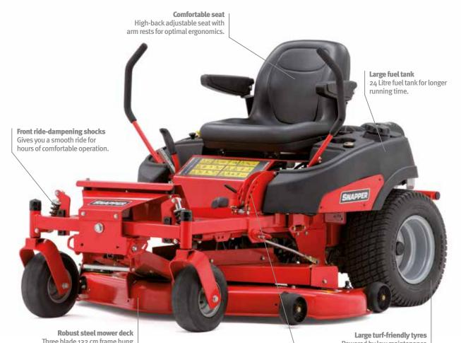
Three blade 132 cm frame hung mower deck.
