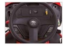
**Ergonomically designed dash board** with hour and fuel meter. cruise control
