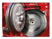
Variable speed disc drive transmission
