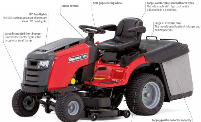
**Large tyres** The large 22" tyres provide superior traction in order to protect your turf. Large 350 litre collector capacity The 350 litre bag features an ergonomic lever to empty the bag without leaving your seat.
