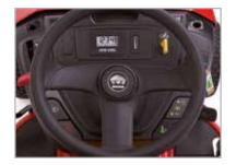
Mini Dash with hour meter, battery voltage and maintenance reminder
