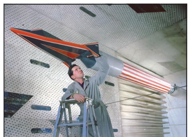
A model of the Boeing Dyna-Soar is tested in a transonic wind tunnel at then-Arnold Engineering Development Center in 1959. It was 70 years ago this month that President Harry Truman signed into law the bills that allowed for the establishment of what would become Arnold Engineering Development Complex. (U.S. Air Force photo)
