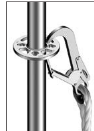
Fig. 10: Attachment in small or large hole of the rosette is possible. (only valid for Allround Scaffolding steel – not for aluminium)
