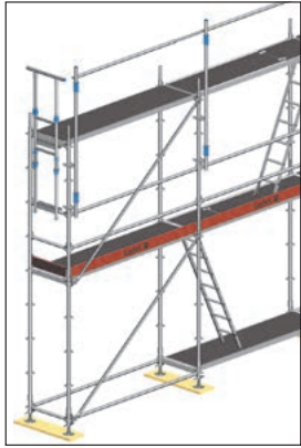
Fig. 15: Assembly of end advance guardrail
