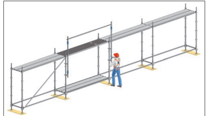
Fig. 18: Use of the advance guardrail in the access bay
