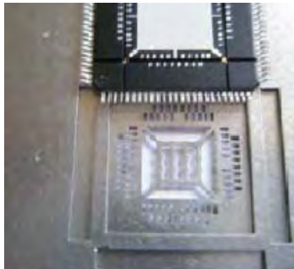
Figure 5 • Example Stencil for Inner Leads Paste Printing
