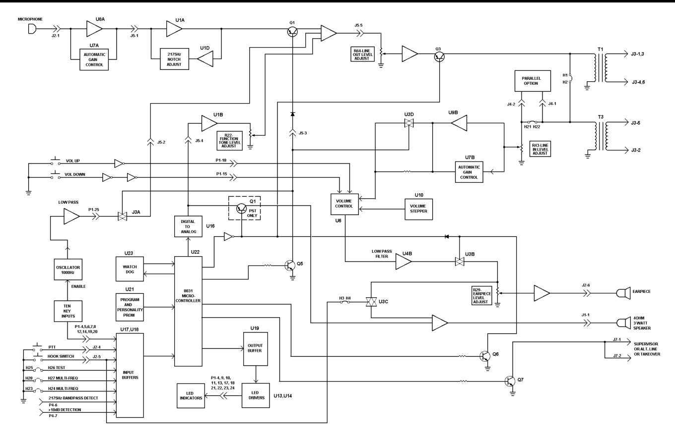
Figure 3 - EDACS RCN Block Diagram
