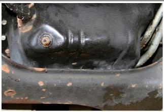
Step 35: Unbolt the starter. Shouldn't have to remove wiring, it just needs to be loose
