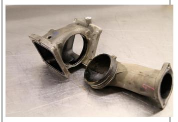
**Step 16:** (A) Remove the Y-bridge studs using 2 nuts. (B)Relocate and install them into the front location of the intake runners
