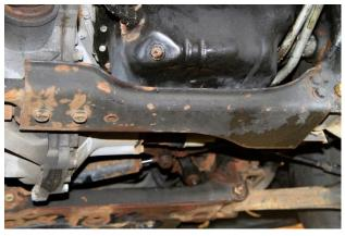
**Step 34:** Remove the oil pan. Clean the gaskets off of both sealing surfaces.
