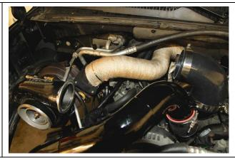
**Step 43:** Install the supplied fitting into the font passenger side of the block and then route the hose from the block fitting up to the oil inlet of the turbo. **(Do not use Teflon tape)**
