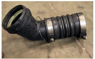
**Step 9**: (A) Remove the 2 bolts in the valve covers on the crank case breather tubes (both sides of the engine) then remove the clamp around the turbo mouth piece. (B) Disconnect the intake air temp sensor and remove. Remove the mouth piece. (Save the mouth piece clamp)
