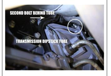
**Step 12:** (A) Remove the factory turbocharger down pipe. (B) Also remove the up pipes going from the manifold to the rear of the turbo.
