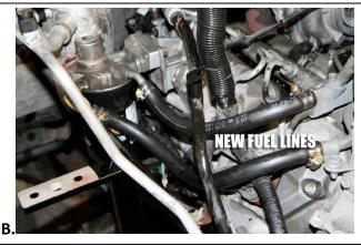
**Step 29**: (A) Install the supplied breather fittings into each valve cover. (B) Then route the hose toward the ground.
