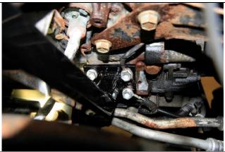
**Step 26:** Remove the dip stick mounting bracket. Cut the end of the bracket off as shown for better clearance. Then reinstall
