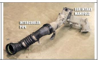
**Step 8:** Loosen the 2 lower intercooler boot clamps and remove the boot off the upper piping. (Save the lower elbow, boot, 2 clamps and snap ring)
