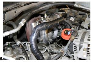
**Step 22**: Remove the passenger side battery cable from the block. Save this cable for reinstallation later on.
