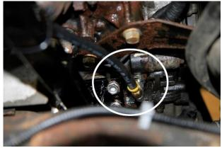
**Step 44:** Reinstall the intake air temperature sensor back into the y-bridge. This sensor is fragile! Take care not to damage the wires or over tighten.
