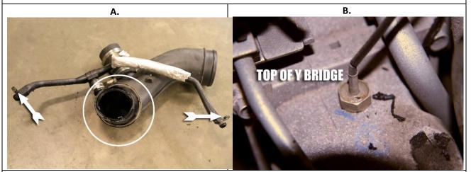
**Step 10:** Remove coolant hoses going to the EGR cooler. Remove the nuts for up pipe going into the EGR cooler. Remove the EGR cooler and EGR valve assemble.
