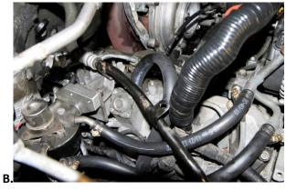
**Step 30:** Install the turbo drain fitting into the turbo mounting bracket. (Be sure to use a thread sealant on the fitting.)
