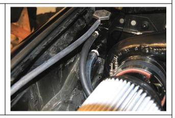
**Step 51:** (A) Install the filter adapter piece. Install the filter. Position everything so there is good clearance on the filter. (B) Then install the MAF sensor. This has to go in a certain way **(the element needs to face the filter.)**
