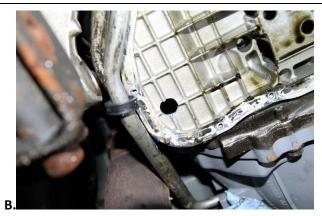
**Step 37:** Once its drilled then thread the hole from the **TOP** of the oil pan using a 3/8-18 NPT tap. Make sure to clean any metal shavings off of any surrounding internal areas.
