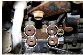
**Step 25**: Install the turbo mounting bracket to the engine block using the 4 bolts supplied. (make sure to put the 2 ground wires back onto the 2 mounting bolts.)
