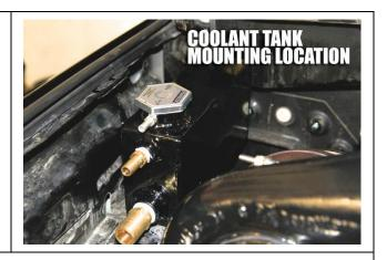
**Step 50:** Install the new supplied coolant lines from your coolant tank to your factory hoses.
