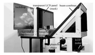
Figure 1. Setup of a beam-combiner with an LCD mask.
