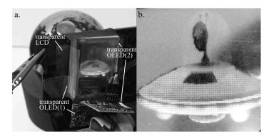
Figure 13a,b. Images of dual-layer transparent OLED with LCD mask. a. Stacked dual-layer transparent OLED with transparent LCD panel, b. Dual-layer image with depth anti-aliasing and mask
