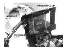
Figure 11. Setup of transparent OLED with LCD mask.
