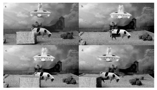
Figure 3a,b,c,d. Images from a beam-combiner with LCD mask, foreground object and phantom masks. a. Pepper's Ghost with LCD mask and a foreground object, b. Foreground object removed with phantom object present, c.Foreground object w/phantom object, d. Another view of beam-combiner with LCD mask, foreground object and phantom masks
