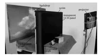
Figure 6. Setup of scrim projection with LCD mask.
