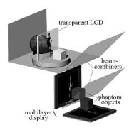
Figure 4. Setup of beam-combiner with multilayer display and LCD masks.
