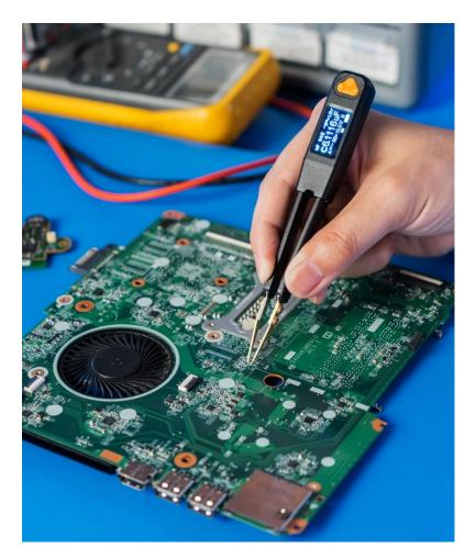
The LCR Pro1 integrates a pair of tweezers like probes and a LCR meter into one compact, lightweight, battery powered device. It is an all-in-one miniature device that provides a simple and efficient solution for not only measuring SMD components, but also making in-circuit debugging.
