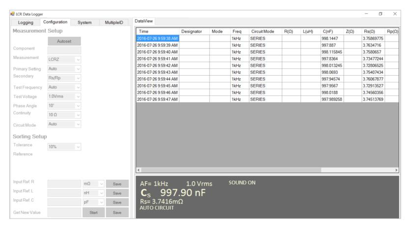
The LCR Data Logger is an easy-to-use Windows based software that is downloadable for free from our website. It provides an intuitive user interface on PC to remote control the Pro1 that is connected to PC via the LCR Link1. It configures the Pro1 parameters and logs the measurement results to an Excel spreadsheet.
