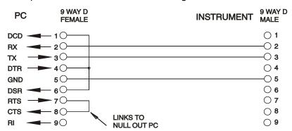
Most commercial cables provide these connections.
