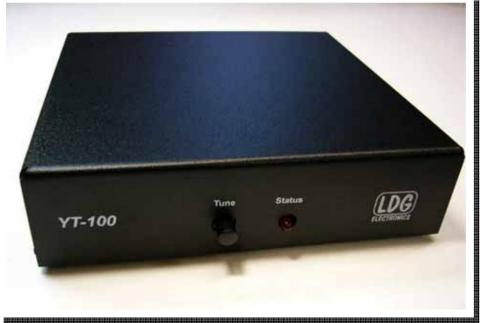
• **Tune Button:** Initiates either a memory tune or a full tune, and also toggles the tuner between "active" and "bypass" modes.
