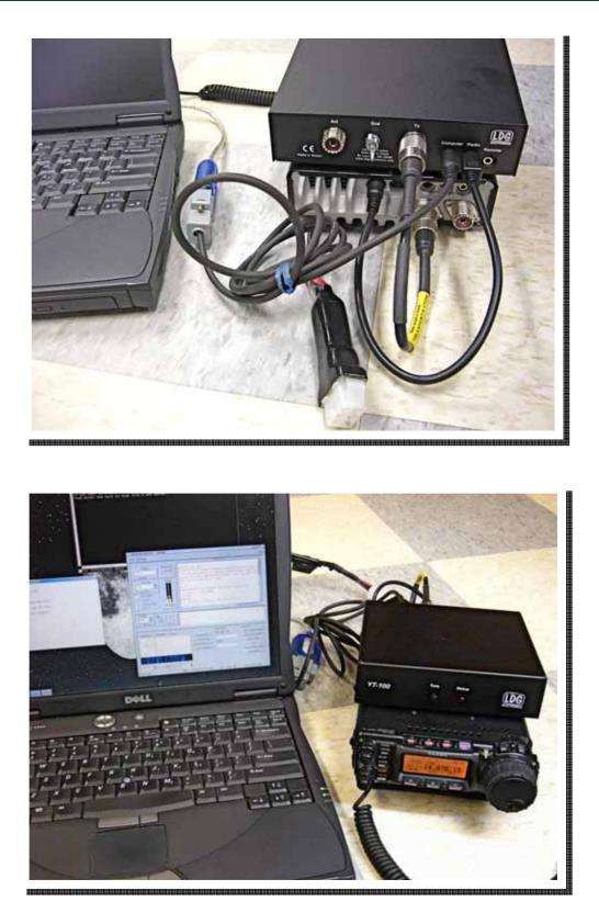
The YT-100 monitors the **Computer** port for activity before beginning any tuning cycle. Only when the CAT line is idle for a period of time will the YT-100 take over control of the CAT line in order to
