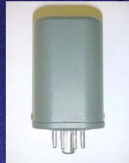
Whisker Short Failed Nuclear Powerplant Relay
