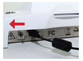
Figure 2-2 Turn Analyzer On
