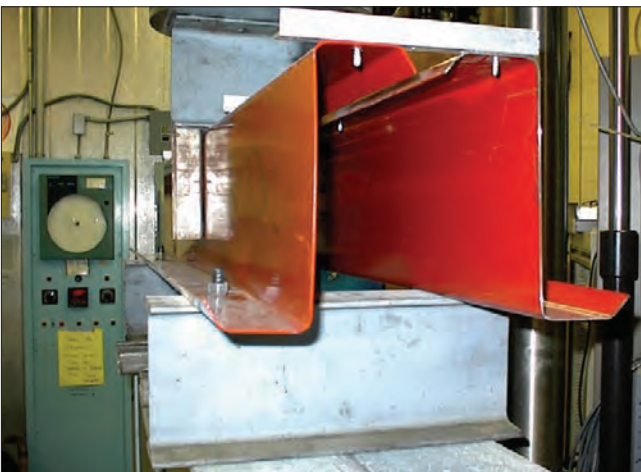
Web crippling tests run by Dr. Roger LaBoube at the University of Missouri-Rolla.
