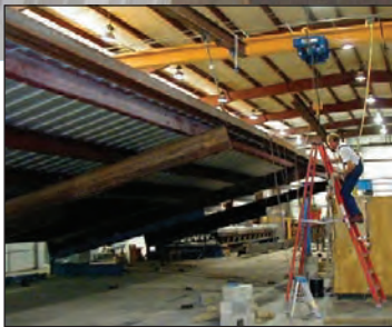
Testing at Virginia Tech to determine purlin roll forces at different roof slopes. MBMA Graduate Fellowship winner Michael Seek is pictured.
