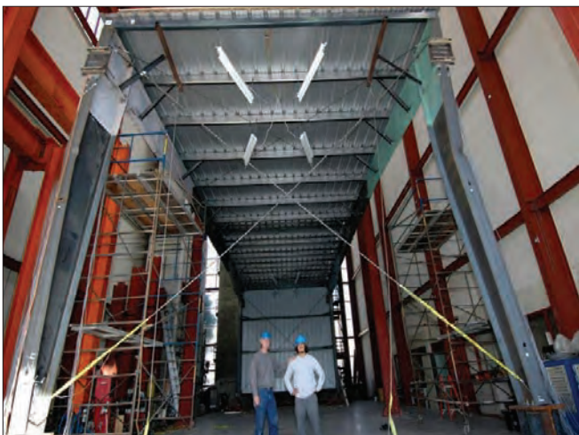
Full-scale seismic loading test at the University of California–San Diego.
