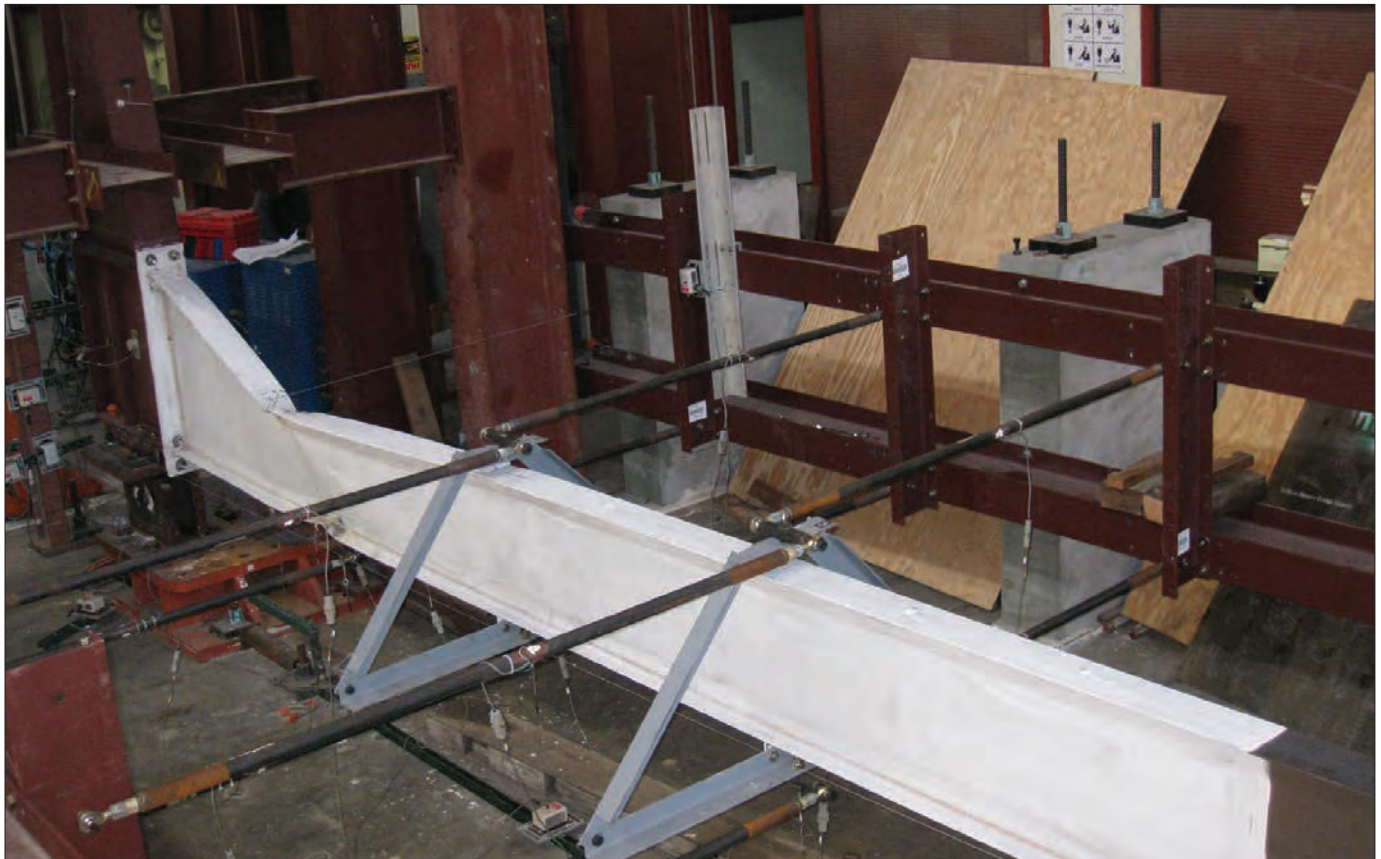
A test that subjects a partial frame of tapered members to a cyclic load to observe the buckling behavior.
