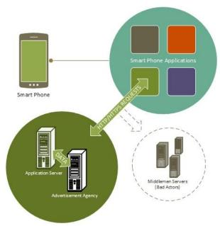
Figure 2 | Communications between smart phone applications and servers
