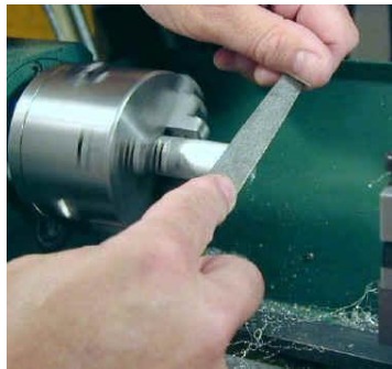
Wrong: left hand reaching over spinning chuck!
