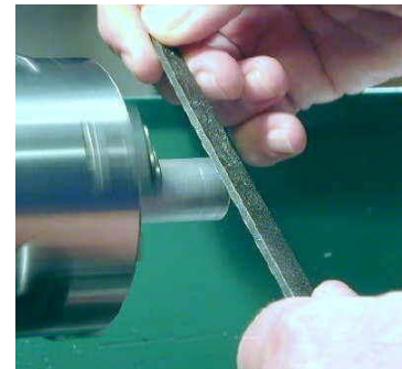
Right - left hand holding tang end of file
