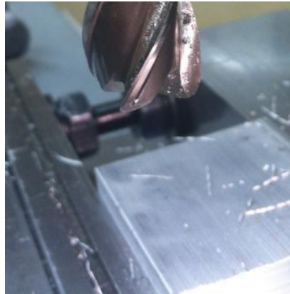
Bolt is placed on the far end to ensure the jaws remains parallel as it clamps the part
