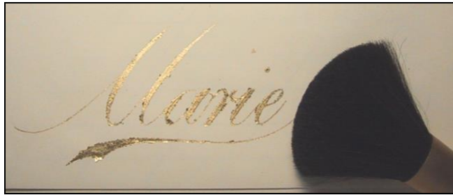
Figure 3: The 23k patent gold leaf was applied using gentle finger pressure. The rule is keep applying the leaf until no more sticks. The image shows the excess gold flash which is removed using a very soft 'Make up' brush to gently remove the flash.
