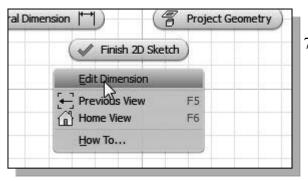
Inside the graphics window, click once with the right-mouse-button to display the option menu. Turn off the Edit Dimension option through the pop-up menu. We will modify all of the dimensions once we are finished with all the necessary editing. 8. The message "*Select Geometry to Dimension*" is displayed in the *Status Bar* area, located at the bottom of the Inventor window. Select the left vertical line as shown below.
