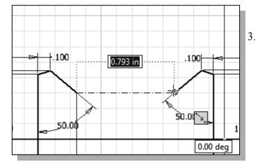
3. Select the endpoint of the longer inclined line on the right as shown.
