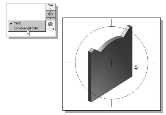
5. Activate the **Constrained Orbit** option by clicking on the associated icon as shown.
