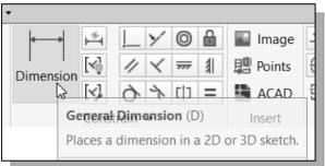
1. Move the cursor to the *Constrain* toolbar area; it is the toolbar next to the 2D *Draw* toolbar. Note the first icon in this toolbar is the **General Dimension** icon. Left-click once on the icon to activate the **Dimension** command. 2. The message "Select Geometry to Dimension" is displayed in the Status Bar area at the bottom of the Inventor window. Select the left vertical line by left-clicking once on the line.
