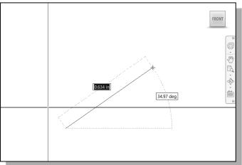
The readout displayed next to the cursor is called the *Dynamic Input*. This option is part of the **Heads-Up Display** option that is new in Inventor. *Dynamic Input* can be used for entering precise values, but its usage is somewhat limited in *parametric modeling*.
