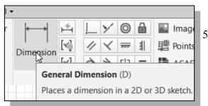
5. Select the **General Dimension** command in the *Constrain* toolbar. The **General Dimension** command allows us to quickly create and modify dimensions.
