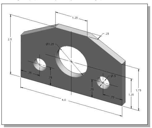
3. **Positioning Stop** (Note the symmetry in the design.)
