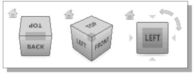
Once the ViewCube is displayed, it is shown in one of the corners of the graphics window over the model in an inactive state. The ViewCube also provides visual feedback about the current viewpoint of the model as view changes occur. When the cursor is positioned over the ViewCube, it becomes active and allows you to switch to one of the available preset views, roll the current view, or change to the Home view of the model.
