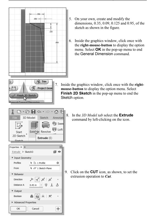
10. Set the *Extents* option to **Through All** as shown. The *All* option instructs the software to calculate the extrusion distance and assures the created feature will always cut through the full length of the model.
