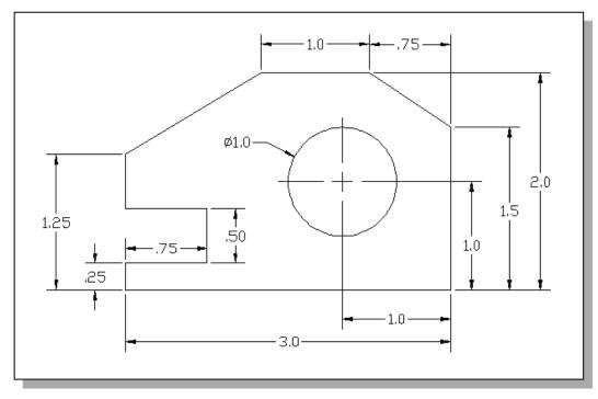
1. Inclined Support (Thickness: .5)
