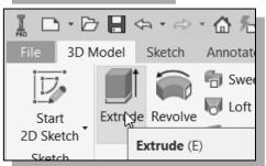
8. In the *3D Model tab* select the **Extrude** command by clicking the left-mouse-button on the icon.
