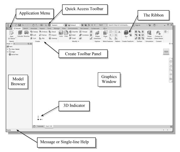
• The *Ribbon* is a relatively new feature in Autodesk Inventor; since the 2011 release the *Ribbon* is composed of a series of tool panels, which are organized into tabs labeled by task. The *Ribbon* provides a compact palette of all of the tools necessary to accomplish the different modeling tasks. The drop-down arrow next to any icon indicates additional commands are available on the expanded panel; access the expanded panel by clicking on the drop-down arrow.
