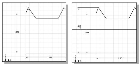
12. Select the bottom horizontal line as the 2<sup>nd</sup> geometry to dimension.
