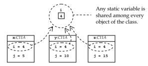
Figure 178: A diagram showing three objects of the C11A class and the values of their instance and class variables
