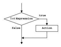
Figure 91: A flowchart associated with an if construct
