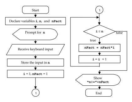
Figure 33: Flowchart of program calculating the factorial of a manuallyinput integer value
