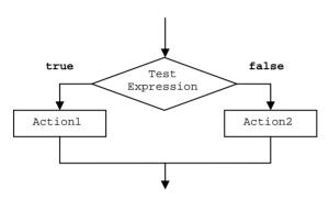
Figure 94: A flowchart associated with an if-else construct
