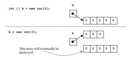
Figure 149: Assigning a new array to a variable
