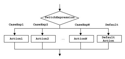
Figure 107: A flowchart representing a switch construct
