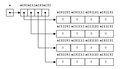
Figure 159: An array of arrays of int
