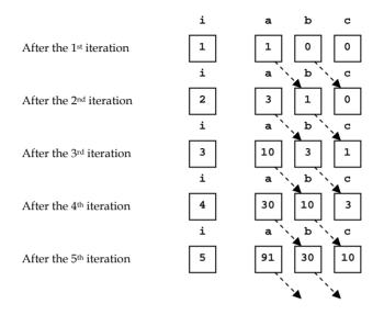
Figure 164: How variables change when the loop keeps iterating
