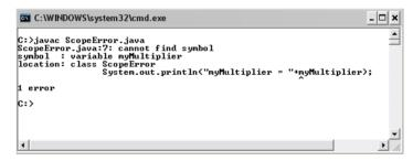
Figure 133: Compilation error due to usage of a variable declared inside a method outside the method
