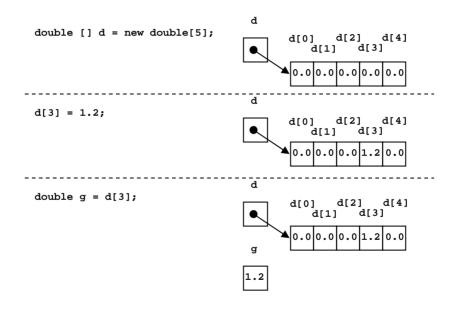
Figure 145: Illustration of accessing an array element
