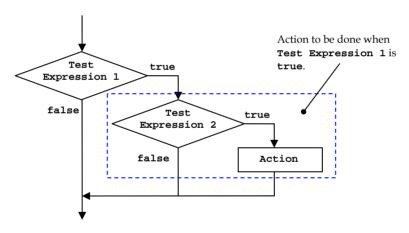
Figure 97: A flowchart associated with a nested if construct
