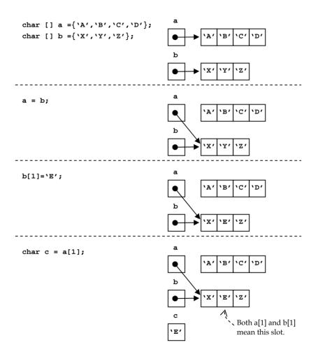
Figure 150: Assigning an array variable to another array variable
