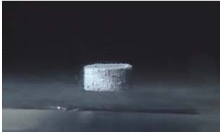
Figure 11. A rare earth magnet levitating above a high-temperature superconductor in a bath of liquid nitrogen
