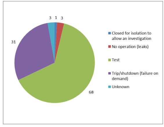
Figure 1: Reasons for valve operation of RESDVs that failed.
