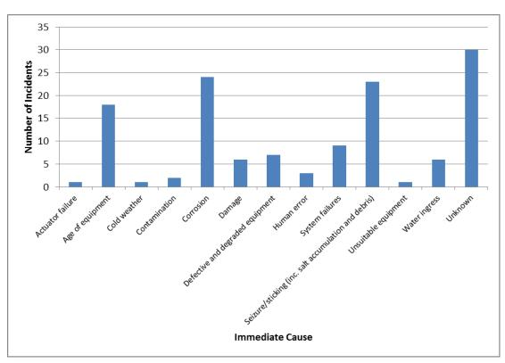
Figure 3: Immediate causes of RESDV failures.
