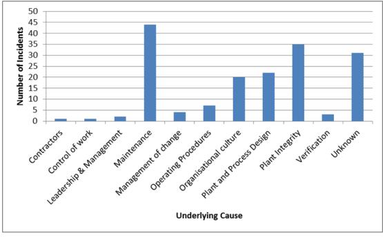
Figure 4: Underlying causes of RESDV failures.
