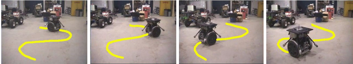
FIGURE 5.3. Segway RMP robot performing the spatial trajectory following task (approximate ground path drawn in yellow).
