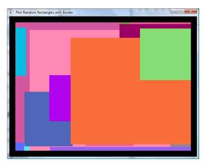
Figure 77 - Setting a border using a clipping rectangle
