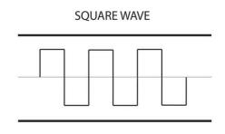
The PC speaker is normally meant to create a square wave via only 2 levels of
