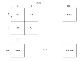
You can view the video display as consisting of a grid of pixels.
