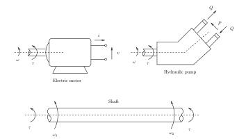
Interconnection: Electrical motor + Shaft + Hydraulic pump
