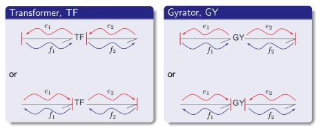
Fixed causality elements Constrained causality elements Preferred causality elements Indifferent causality elements
